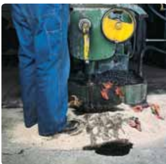
Problem: Leaks and drips create a slippery work floor.
