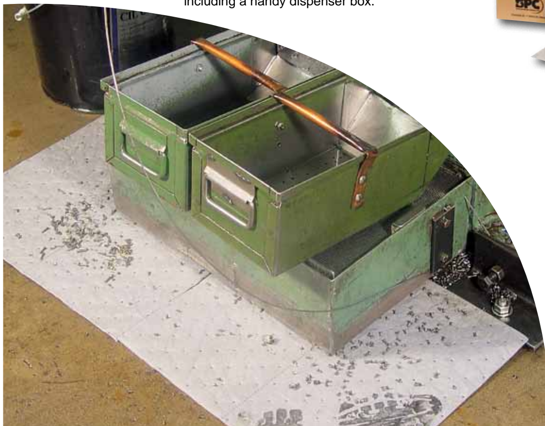
A good general use sorbent to fit around machines to adsorb overspray.
