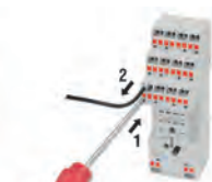
Cable removal with screwdriver
